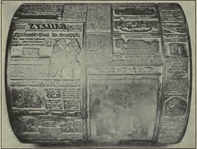
FIG. 8.—Curved plate for rotary newspaper press—produced from matrix shown in Fig. 7.
